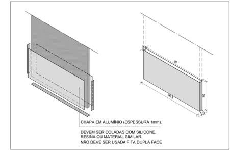
DETALHE CHAPA METÁLICA
